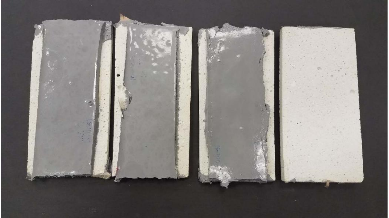
Photo 7 – ASTM C510 Specimens after UV Exposure – No Stain or Color Change
