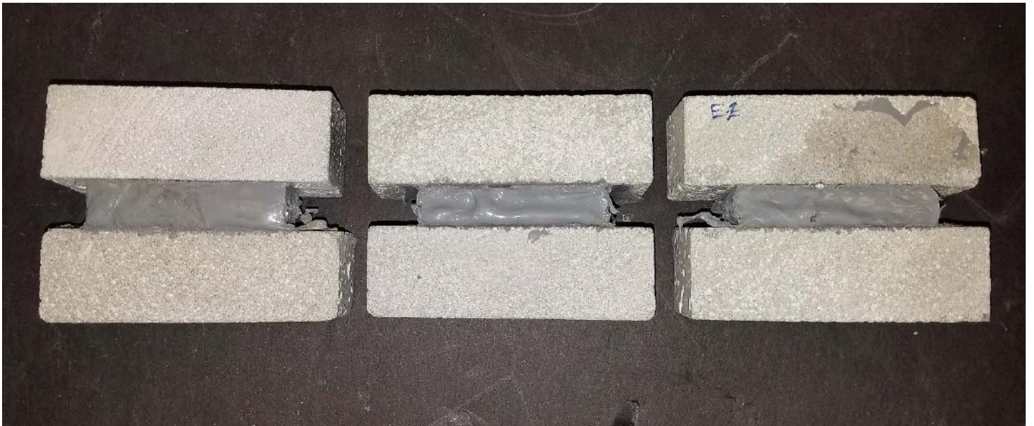
Photo 8 – ASTM C719 Specimens following Extension/Compression Cycles
